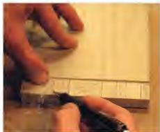
Drafting square. Register a plastic drafting square against the narrow shoulder to divide the "giant tenon" into small tenons.
